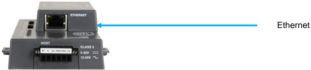
Figure 9: Ethernet port location on the ProtoNode
